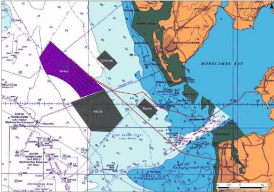
Figure 3.1: Layout for Walney Offshore Windfarm. The array cable routes (black) and the routes of the submarine export cable to the shore at Heysham (top red line).
